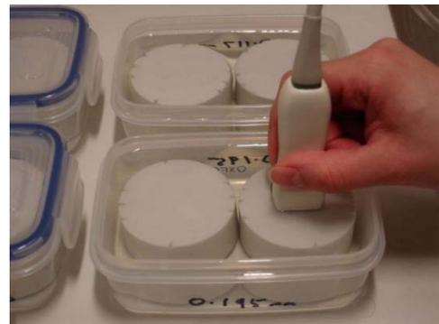
*Figure 2: Image of the modified Edinburgh Pipe Phantom to assess preclinical ultrasound scanners*
